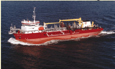
Trailing suction hopper dredges.
