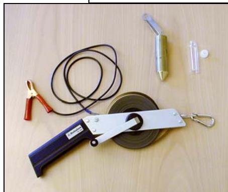
Sample collector with steel measuring tape.
