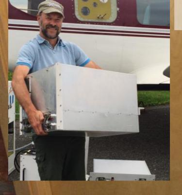
Sulfur sniffer Logging Computer AIS and GPS reciever Calibration gas CO2 sensor SO2 sensor Power converters, TCP -IP 47 kg, 15 A @ 28 V DC 19" dimension
