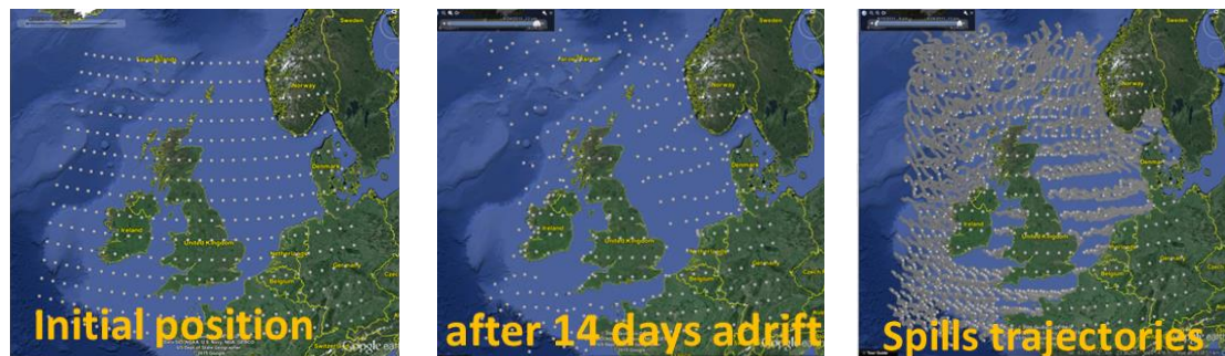
Figure 2 The OSERIT model simulates under realistic met-ocean conditions 14 days drift trajectories of 1955 oil spills initially distributed on a regular lattice covering the whole Bonn Agreement area.
