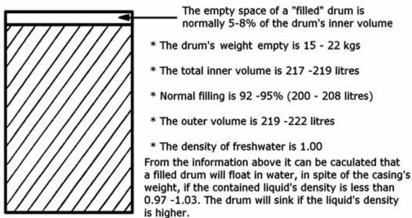
**Figure 2.8.7** Calculating the buoyancy of drums
