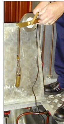
Sample collector with steel measuring tape.
