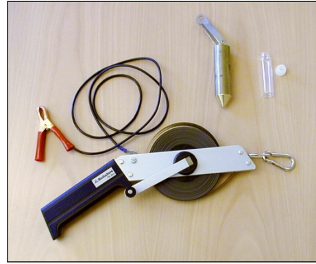
Sample collector with steel measuring tape.
